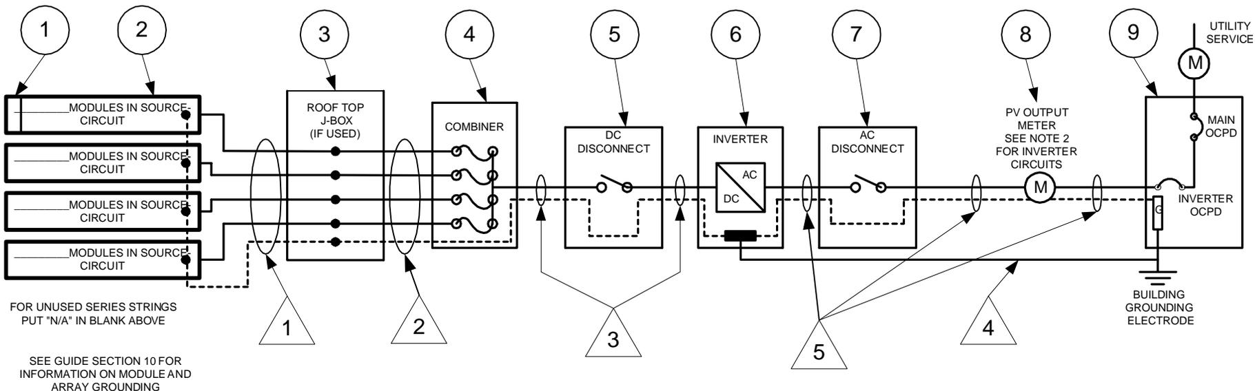
**STANDARD ELECTRICAL DIAGRAM FOR SMALL-SCALE, SINGLE-PHASE PV SYSTEMS**
